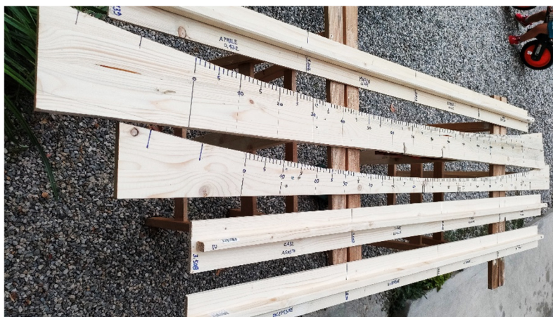
Fig. 12. The arched wooden metric templates with the radius of the tank, used to trace the hour lines.
